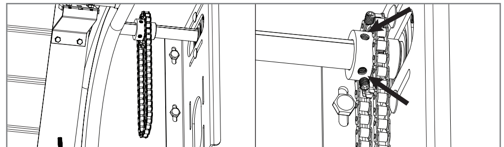
06 - Pull the pinion to the bearing and tighten the two bolts to secure the pinion to the shaft.
